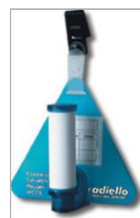
Figure 10 | Tube passif (type Radiello)
