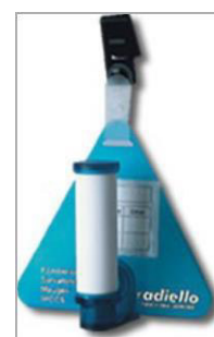
Figure 1 : tube passif (type Radiello)
